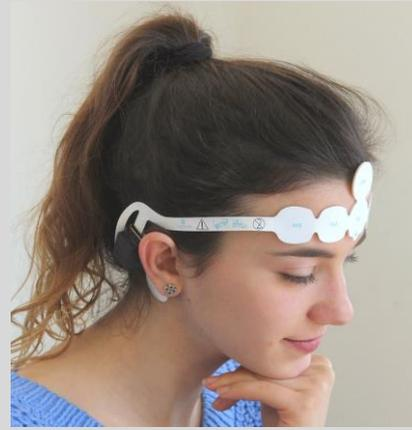
*Bioimpedance and biopotential amplifier BIOPOT for wireless biopotential and bioimpedance monitoring (device behind the ear).*
