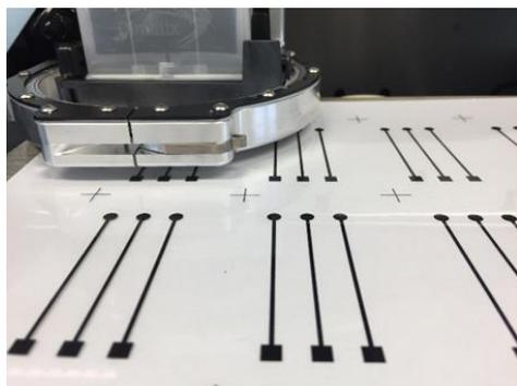
Printed test electrodes (© Fraunhofer IBMT).
